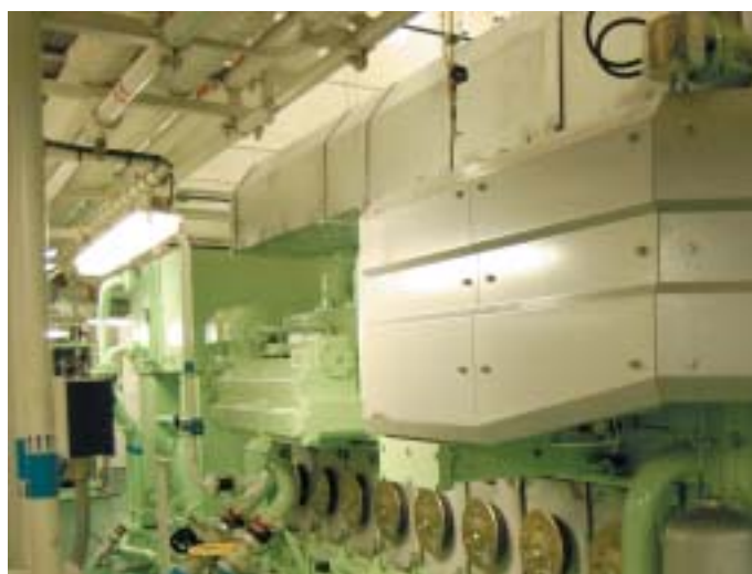
Six Wärtsilä dual fuel engines provide a total of 20.160 kW
