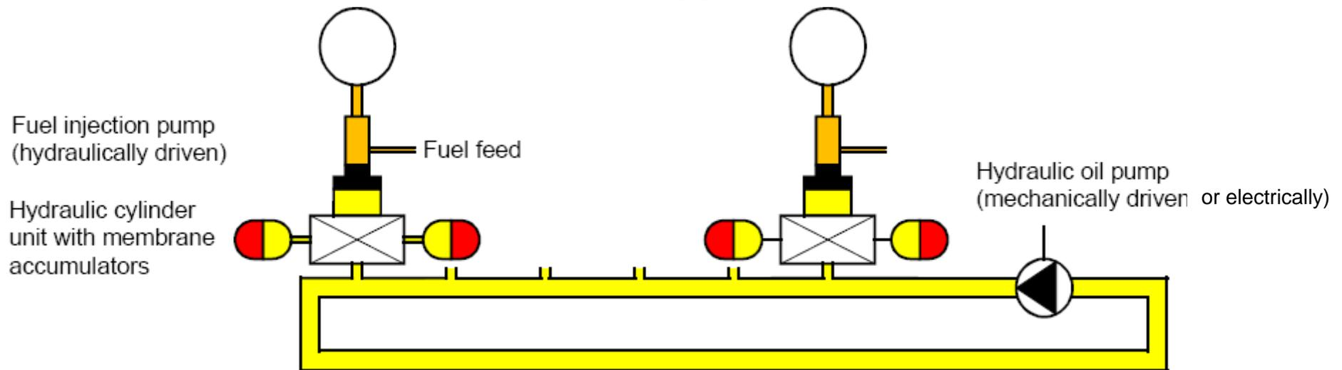
Efficiency loss in the hydraulic system
