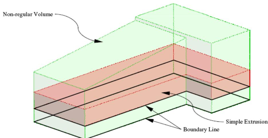
The Boundary Line element defines the footprint or boundary of an architectural component; it is used for quick visualisation in both 2D and 3D views to show the extents of the major architectural component.
