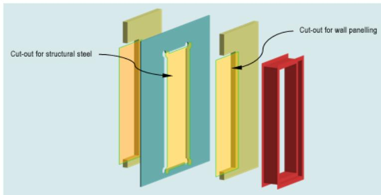
Where a penetrating element is the same shape whatever it is penetrating, there still needs to be two penetrating loops with different purposes even though they are identical.
