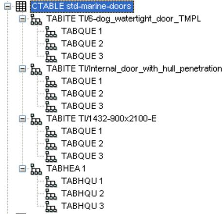
With just a single list of TABITEMS, the Choose form definition would simply be a single column list of tabitem names. The ability to add TABQUESTIONS adds a set of extra columns for the choose forms and enables extra selection criteria to be applied.
