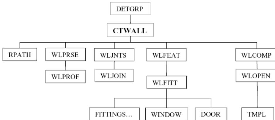
The path of the wall defines the route along which a constant thickness rectangular cross-section is extruded, and this can contain straight and curve segments. The path is similar in concept to the general section (GENSEC) available within the system; however, the extruded cross-section for the wall is not catalogued.
