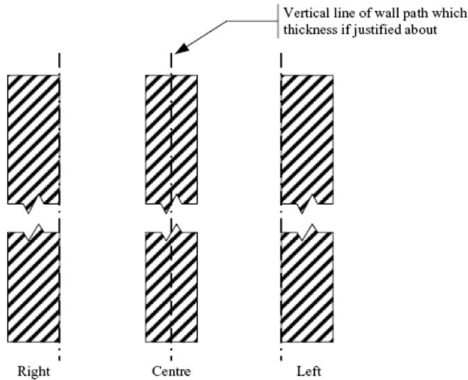
The height of the wall is measured in the vertical; however, it is possible to define an offset angle from the vertical for the wall and the wall thickness is always the distance between the two outer surfaces of the wall, regardless of the angle of the wall.
