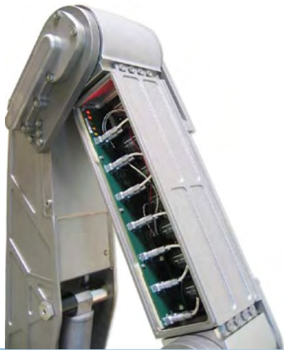
Slave arm electronics are located in the forearm, increasing system reliability and minimizing electrical connections.
