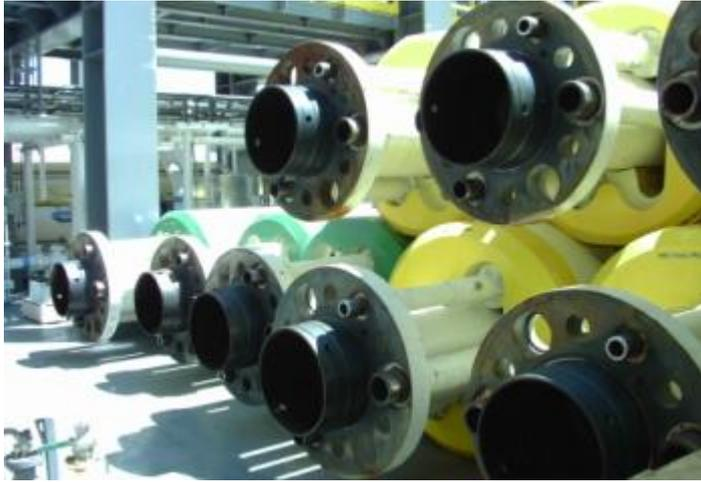
The different color stripes on the risers indicate differing amounts of buoyancy. The idea is to put heavy riser pipe down at the bottom, connected to more buoyant risers above. The buoyancy keeps the entire riser system in more or less neutral buoyancy, so that the drill ship doesn't have to somehow hoist up the huge weight of all that pipe.
