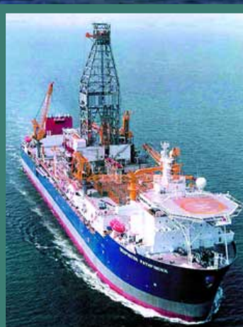
Ship name: Deepwater Pathfinder Owner: Conoco/R&B Falcon Type: Drillship Yard: Samsung
