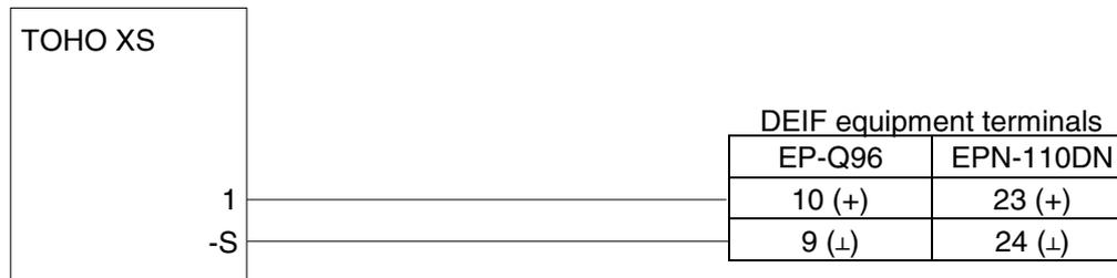
DELOMATIC/PPU/GPC/AGC/BGC output is +/-20mA, so a resistor is needed to convert into 4V DC range:
