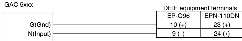
DELOMATIC/PPU/GPC/AGC/BGC output is +/-20mA, so a resistor is needed to convert into 5V DC range:
