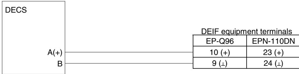
DELOMATIC/PPU/GPC/AGC/BGC output is +/-20mA, so a resistor is needed to convert into 3V DC range:
