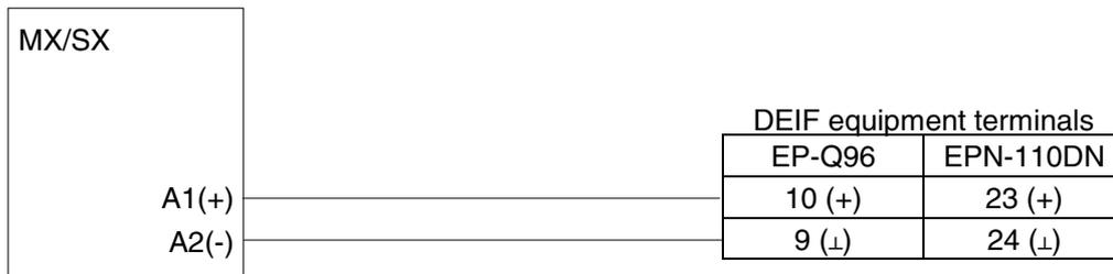
DELOMATIC/PPU/GPC/AGC/BGC output is +/-20mA, so a resistor is needed to convert into 5V DC range:
