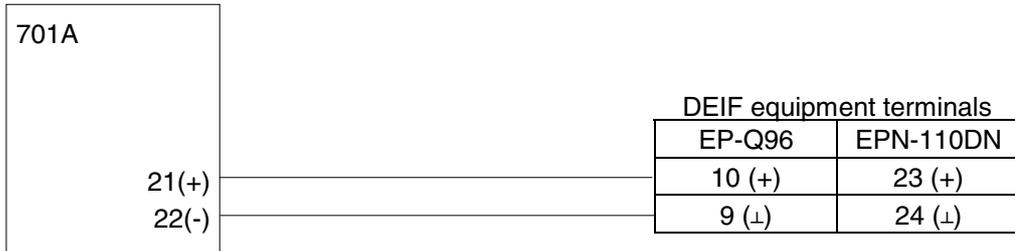
DELOMATIC/PPU/GPC/AGC/BGC output is +/-20mA, so a resistor is needed to convert into 2.8V DC range:
