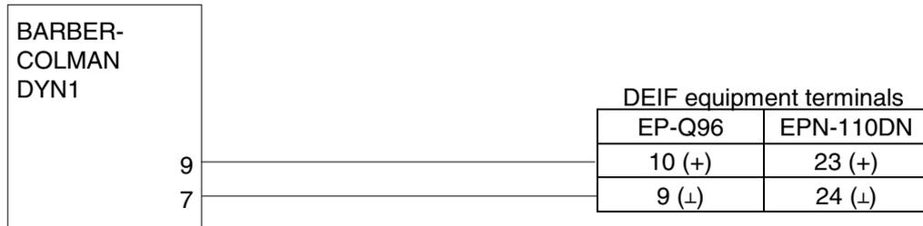
DELOMATIC/PPU/GPC/AGC/BGC output is +/-20mA, so a resistor is needed to convert into 2V DC range:
