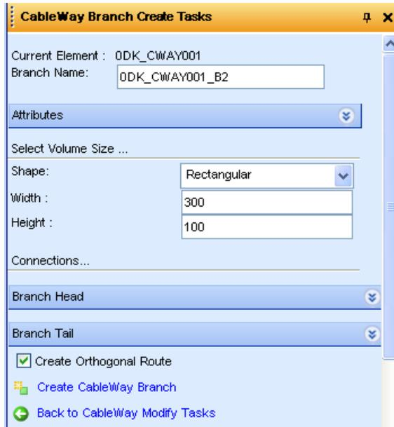
This form allows the user to create and automatically route a cableway branch.
