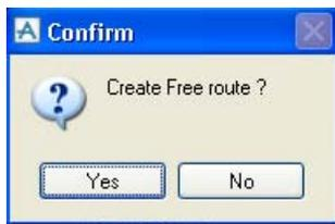
Selecting the **Yes** option routes the cable between the two points and displays the **Modify Free Point** form, which allows the user to modify a route point. Refer to [Modifying a Route Point](#).
