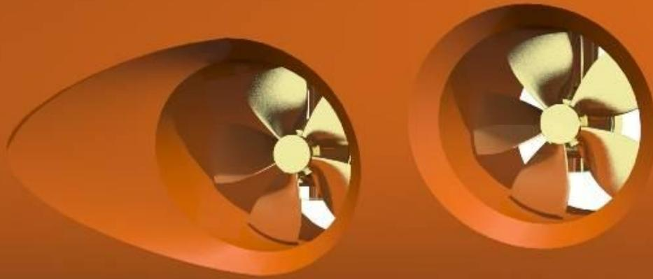
The water flow disturbance from openings to bow thruster tunnels and sea chests can be high. It is therefore beneficial to install a scallop behind each opening. Alternatively a grid that is perpendicular to the local flow direction can be installed. The location of the opening is also important.
