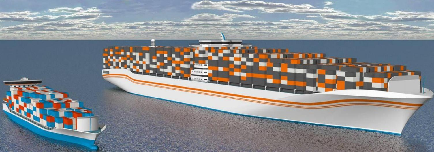
A larger ship will in most cases offer greater transport efficiency – “Efficiency of Scale” effect. A larger ship can transport more cargo at the same speed with less power per cargo unit. Limitations may be met in port handling.
