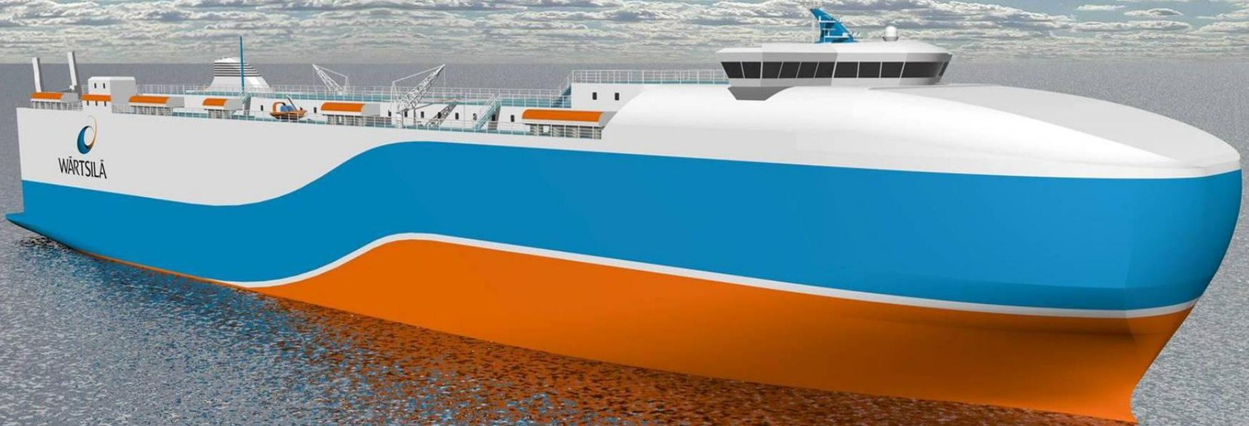
Minimising the use of ballast (and other unnecessary weight) results in lighter displacement and thus lower resistance. The resistance is more or less directly proportional to the displacement of the vessel. However there must be enough ballast to immerse the propeller in the water, and provide sufficient stability (safety) and acceptable sea keeping behaviour (slamming).
