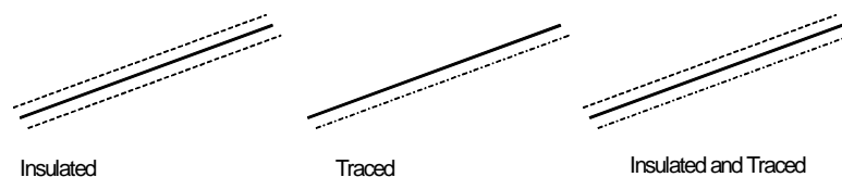
Figure 9.5. Insulated and traced piping
