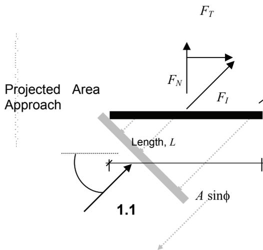
A second approach is to calculate the wind force normal to the member,  $F_N$ , using the normal component of wind pressure,  $\frac{1}{2} \rho V^2$ , projected along the length of the member. For this "Projected Pressure Approach"  $F_N$  will be a function of  $V^2 A \sin \phi$  while  $F_T \cong 0$ . Hence,  $F_I = f(V^2 A \sin^2 \phi)$  and  $F_C = f(V^2 A \sin \phi \cos \phi)$ .
