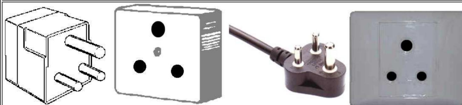
This plug resembles the Indian type D plug, but its pins are much larger. Type M is rated at 15 amps. Although type D is standard in India, Sri Lanka, Nepal and Namibia, type M is also used for larger appliances. Some sockets over there can take both type M and type D plugs.
