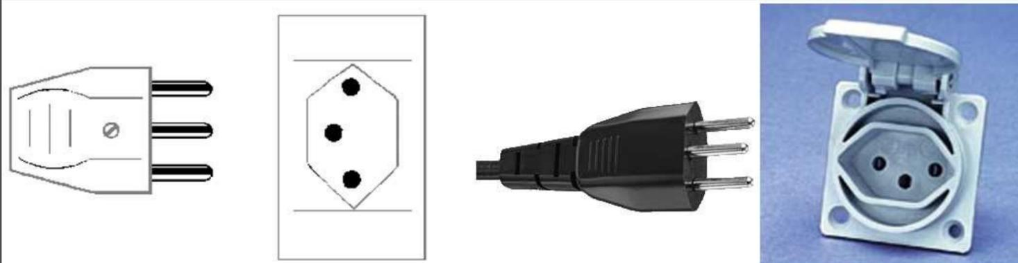
Switzerland has its own standard which is described in SEC 1011. This plug is similar to C, except that it has the addition of a grounding pin. This connector system is rated for use in applications up to 10 amps. Above 10 amps, equipment must be either wired permanently to the electrical supply system with appropriate branch circuit protection or connected to the mains with an appropriate high power industrial connector.
