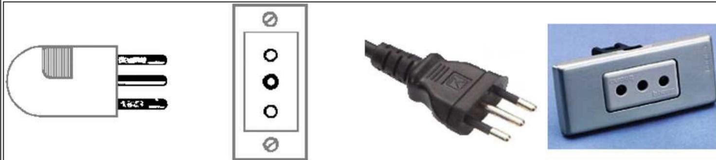
The Italian grounded plug/socket standard, CEI 23-16/VII, includes two styles rated at 10 and 16 amps. They differ in terms of contact diameter and spacing, and are therefore incompatible with each other. The plugs are similar to C except that they are earthed by means of a centre grounding pin. Because they can be inserted in either direction at random, they are unpolarised. A type C plug fits perfectly into a type L socket.
