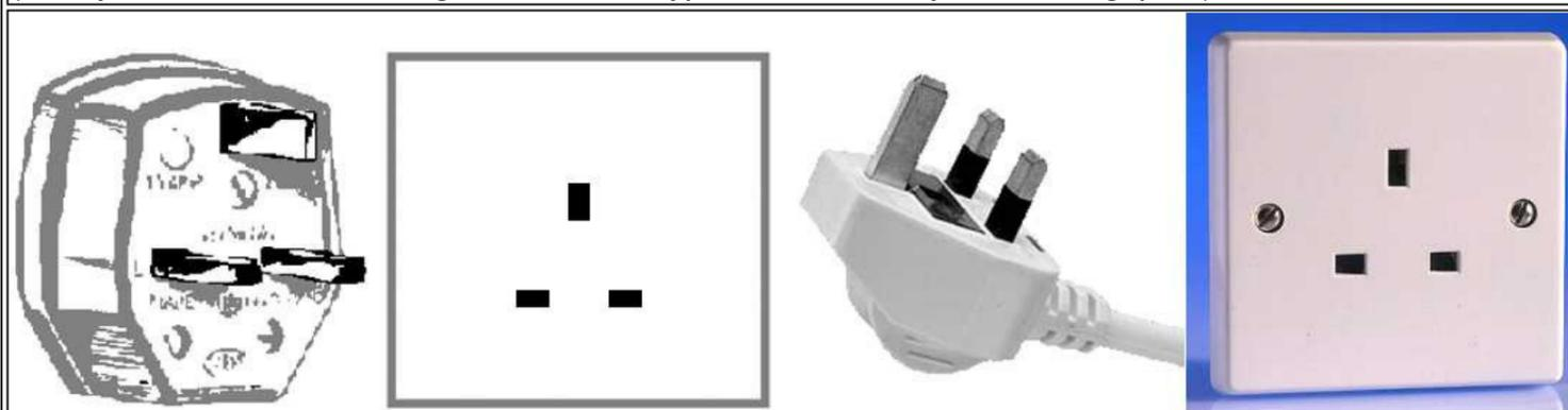
This plug has three rectangular prongs that form a triangle. British Standard BS 1363 requires use of a three-wire grounded and fused plug for all connections to the power mains (including class II, two-wire appliances). British power outlets incorporate shutters on line and neutral contacts to prevent someone from pushing a foreign object into the socket.
