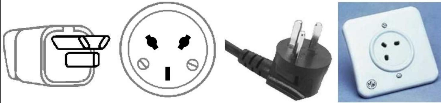
This plug, defined in SI 32, is unique to Israel. It has two flat prongs like the type B plug, but they form a V-shape rather than being parallel like B plugs. Type H plugs have got a grounding pin as well and are rated at 16 amps. Type H sockets are so shaped as to accommodate type C plugs as well. The slots for the non-grounded prongs have widenings in the middle specifically to allow type C prongs to fit in.
