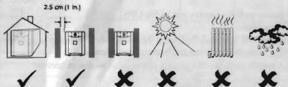
Install the UPS in a protected area that is free of excessive dust and has adequate air flow. Do not operate the UPS where the temperature and humidity is outside the specified limits.
