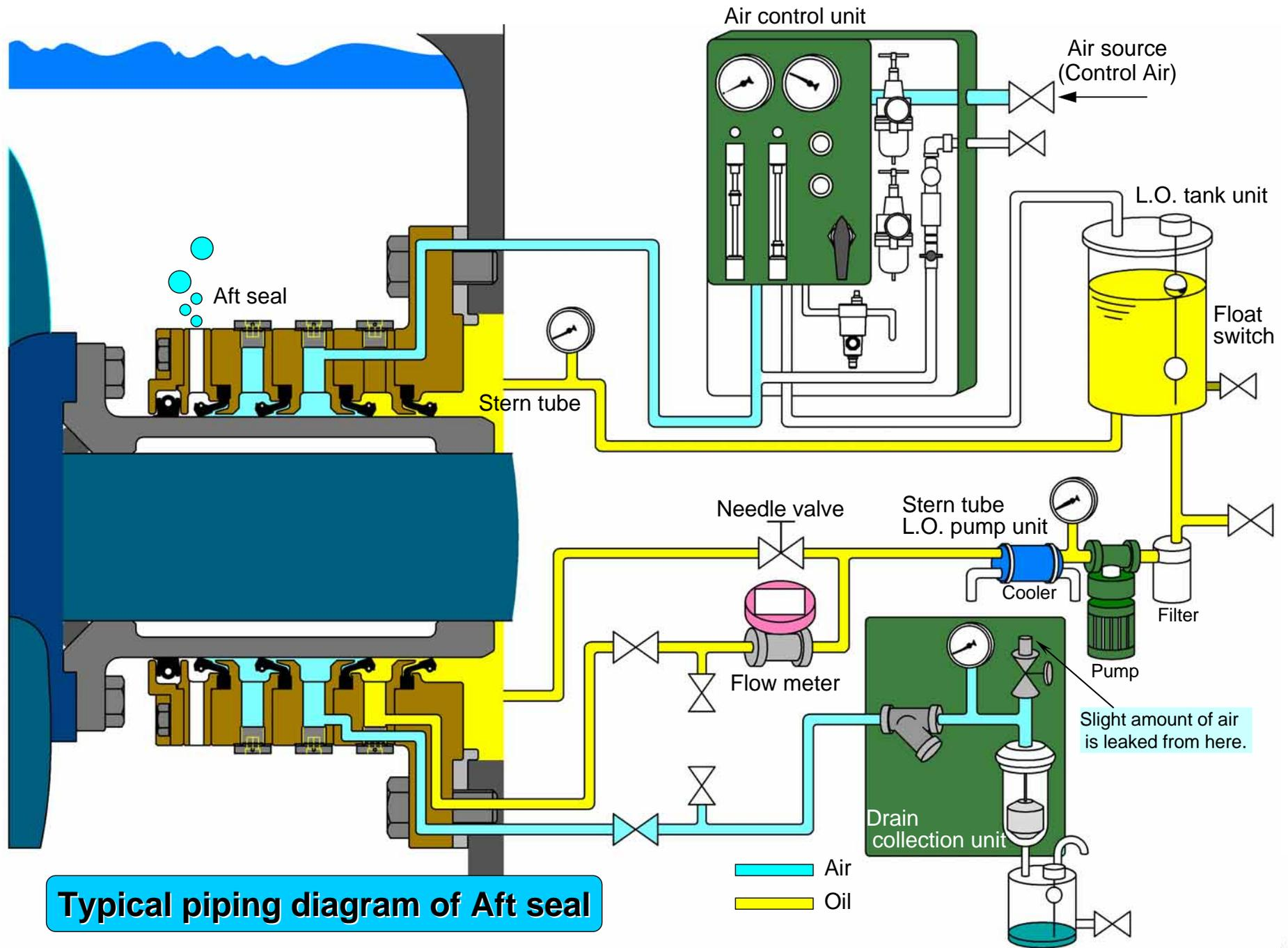
**Typical piping diagram of Aft seal**
