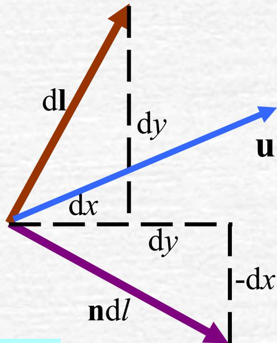
$$\psi(x, y) = \int_{M_0(x_0, y_0)}^{M(x, y)} -u_y dx + u_x dy$$
