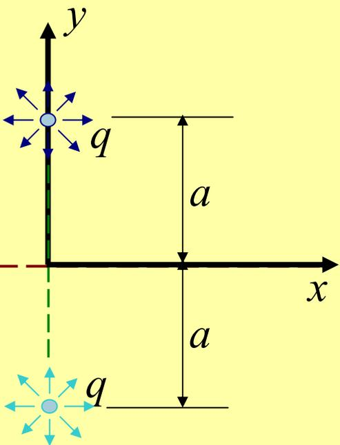
$$\varphi = \frac{q}{2\pi} \left( \ln \sqrt{x^2 + (y-a)^2} + \ln \sqrt{x^2 + (y+a)^2} \right)$$
