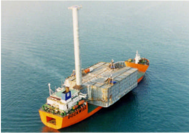
Figure 9: Dry transport of ballasted tank
