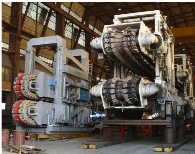
Figure 5 - Side by side comparison between old (right) and new tensioner (left)
