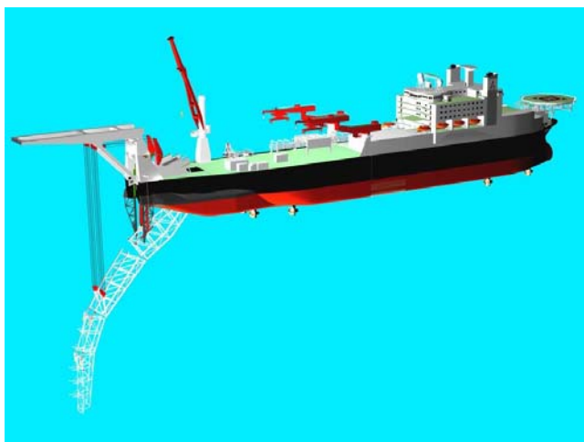
Figure 3 – Overview of stinger and stinger hang-off frame
