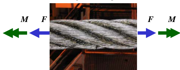
Figure 8 - Stranded wire rope: tension induced torque.
