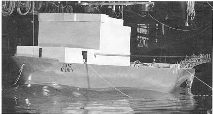
Figure 5 Model tests at MARIN; scale 1:42
