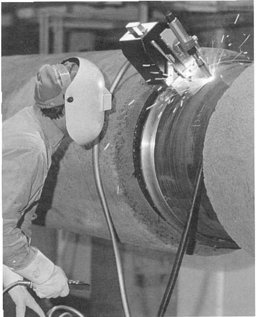
Figure 12 Phoenix automatic welding system
