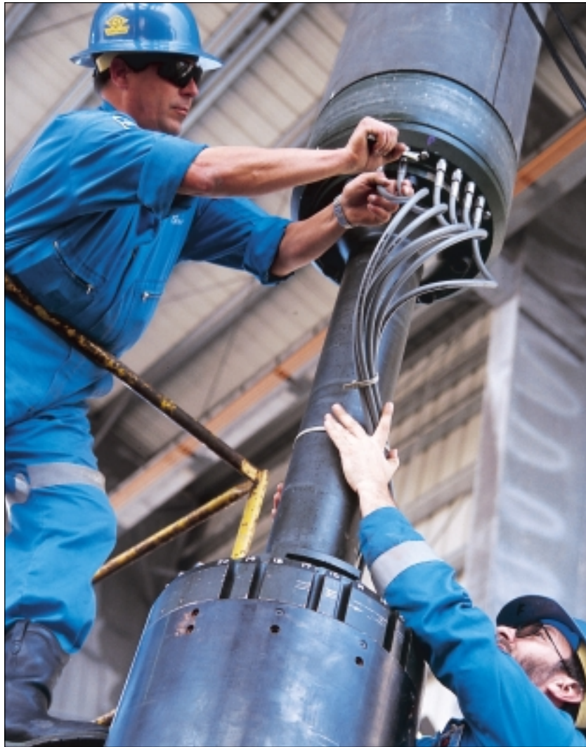
^Engineers assembling a SenTREE7 tool for testing at the Schlumberger Reservoir Completions center.
