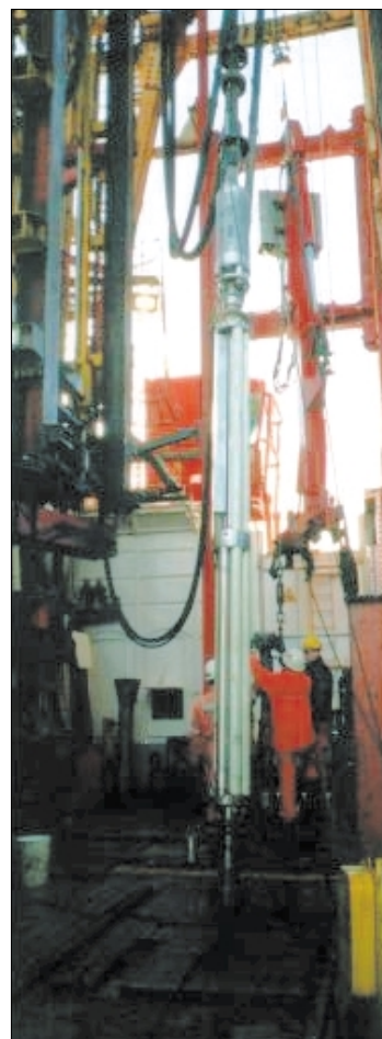
▲ The SenTREE3 tool with electrohydraulic control used for testing the Barden field in the Norwegian North Sea.
