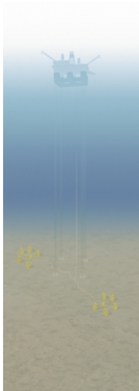
^ Multiple trees. A group of five subsea production trees is linked to a manifold, where flow is collected at a single station before continuing to surface. A second group of five subsea water-injection wells is in the background.
