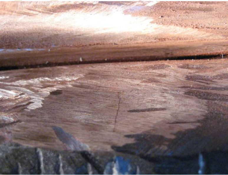
transverse crack
