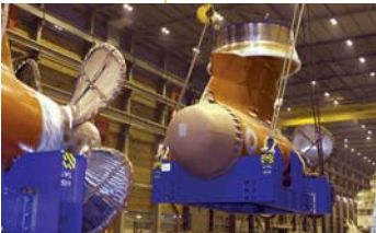
One-lift mounting of Azipod® unit
