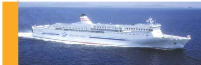
Akashia and Hamanasu are the largest and fastest ferries in Japan and the first vessels to take advantage of the new CRP Azipod® propulsion system.
