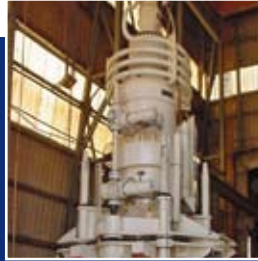
LMRP with FlexLoops and FlexJoint® installed
