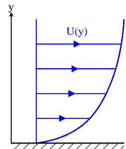
The single most popular type of turbulence closure is called an *eddy-viscosity model* (EVM) which, by direct analogy with the viscous stress, assumes *stress proportional to rate of strain*:
