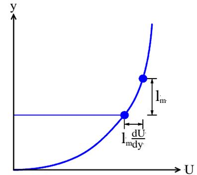
The specification of the *mixing length*  $l_m$  depends on the type of flow.
