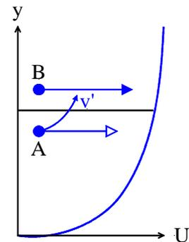
In both cases,  $-\rho u'v'$  is positive and, *on average*, tends to reduce the momentum in the upper fluid or increase the momentum in the lower fluid. Hence there is a net transfer of momentum from upper to lower fluid, equivalent to an additional mean stress.
