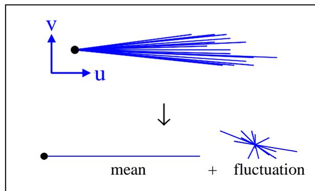
Mean and fluctuating part are denoted by either an overbar (  $\bar{\quad}$  ) and a prime (  $\prime$  ):
