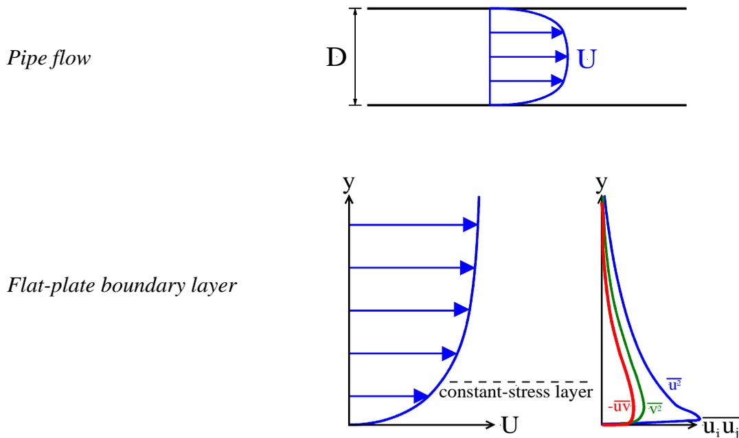
The presence of a solid boundary leads to flow behaviour and turbulence structure very different from free turbulent flows.
