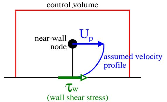
In the finite-volume method, various quantities are required from the wall-function approach. Values may be fixed on the wall ( $w$ ) itself or by forcing a value at the near-wall node ( $P$ ).
