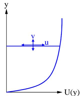
Actually, in *simple shear* flows, this is not a problem, since the shear-stress gradient is the only dynamically-significant term in the mean momentum equation. However, it is indicative of more serious problems in *complex* flows (those for which more than one stress component is dynamically significant).
