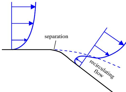
Although its influence in much of the flow is tiny, the small regions (of large velocity gradients) where viscosity is important can have global effects. For example, it is the viscous boundary layer required to satisfy the non-slip condition that is responsible for *flow separation* in an adverse pressure gradient, whilst for erodible boundaries the surface shear stress is responsible for sediment suspension.
