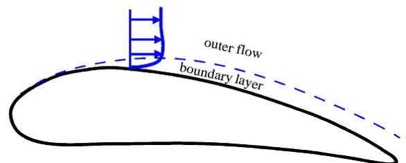
The boundary-layer hypothesis is OK if the boundary layer is thin, slowly-developing and doesn't separate. Using a potential-flow method in the outer layer offers considerable computational savings. However, matching-type calculations are seldom used in *general-purpose* codes because:
