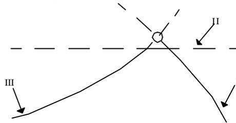
**Range III:** In the low load range the pressure rise is calculated as a reduction proportional to the load. This means that fixed control has been introduced in which the pressure rise is controlled as a function of the engine speed (rpm) and fuel pump index.
