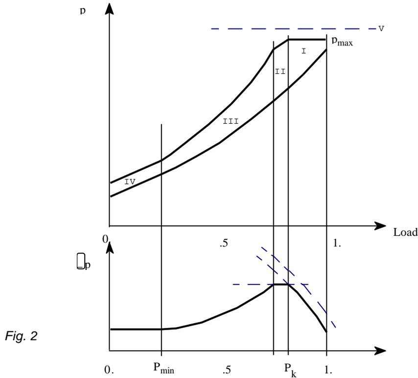
**Range I:** The pressure rise is a controlled variable dependent on the scavenge air pressure, and is calculated as follows:
