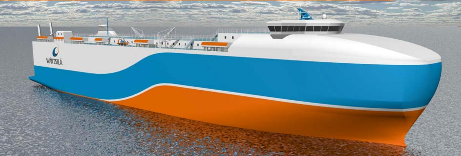
Minimising the use of ballast (and other unnecessary weight) results in lighter displacement and thus lower resistance. The resistance is more or less directly proportional to displacement of the vessel. However there is need to have enough ballast in order to immerse the propeller in the water, sufficient stability (safety) and acceptable sea keeping behaviour (slamming).
