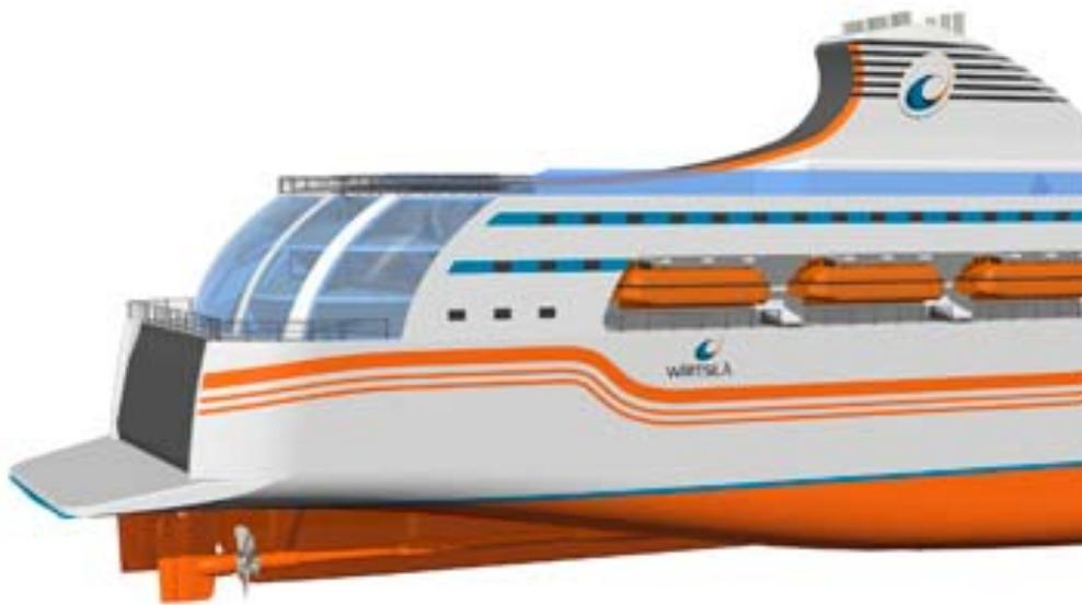
Ducktail is basically a lengthening of the aft ship. It is usually 3-6 meters long. Its basic idea is to lengthen the effective waterline and make the wetted transom smaller. This has positive effect on the resistance of the ship. In some cases best results are achieved when ducktail is used together with Interceptor.
