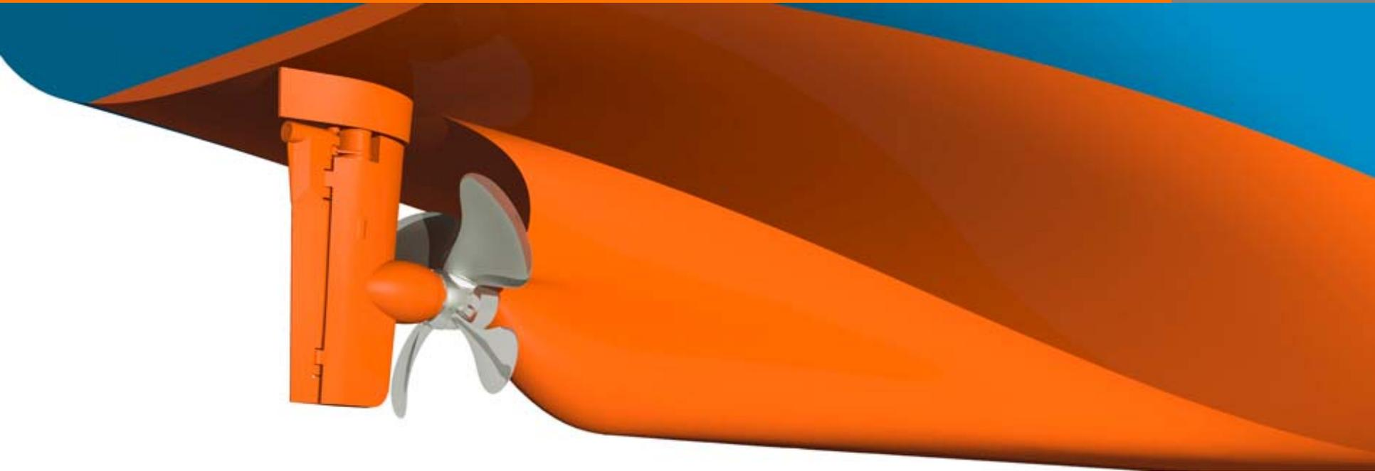
The skeg should be designed to direct the flow evenly to the propeller disk. At lower speeds it is typically beneficial to have more volume on the lower part of the skeg and as thin as possible above the propeller shaftline. At the aft end of the skeg the flow should be attached to skeg, but with as low flow speeds as possible.
