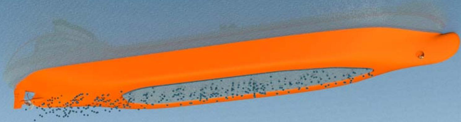
Compressed air is pumped into a recess in the bottom of the ship's hull. The air builds up a "carpet" that reduces the frictional resistance between the water and the hull surface. This reduces the propulsion power demand. The challenge is to ensure that the air stays below the hull and does not escape. Some pumping power is needed.
