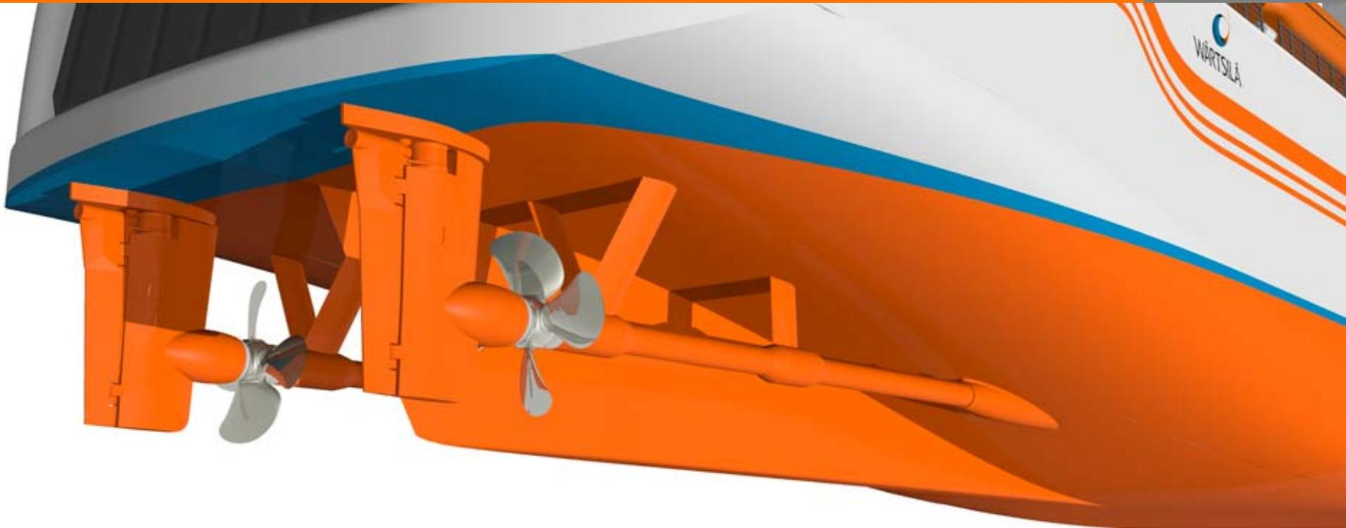
Shaft lines should be lined in streamline direction. Brackets should have a streamlined shape. Otherwise the resistance will increase and the flow to propeller is disturbed.
