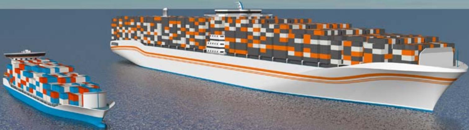
A larger ship will in most cases offer greater transport efficiency – “Efficiency of Scale” effect. A larger ship can transport more cargo at the same speed with less power per cargo unit. Limitations may be met in port handling.
