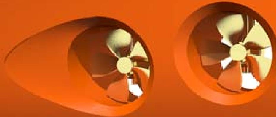
The water flow disturbance from openings to bow thruster tunnels and sea chests can be high. It is therefore beneficial to install scallop behind each opening. Alternatively a grid that is perpendicular to the local flow direction can be installed. The location of the opening is also important.
