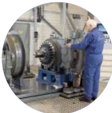
At the test centre the new winches are tested and approved. It is also used for testing and calibration of winches after repairs.
