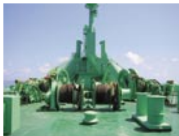
FAR LEFT Arctic Lady and LEFT & BOTTOM Berge Boston , two LNG carriers equipped with Rauma Brattvaag LP hydraulic deck machinery.
