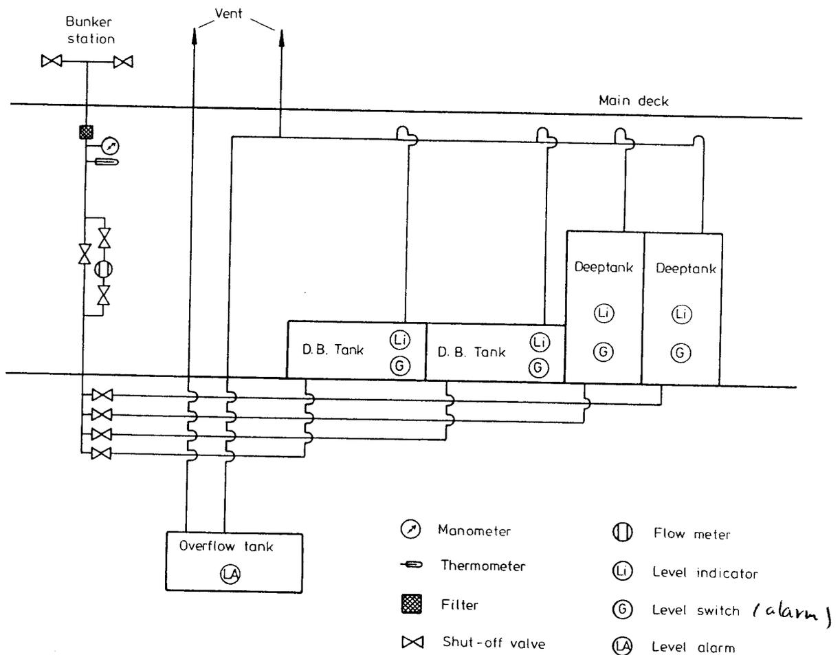
Fig. 1 Fuel Oil Overflow System of Group I
