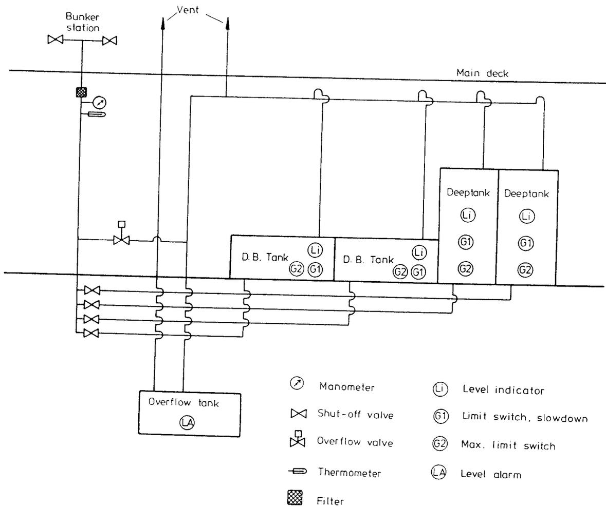
Fig. 2 Fuel Oil Overflow System of Group II
