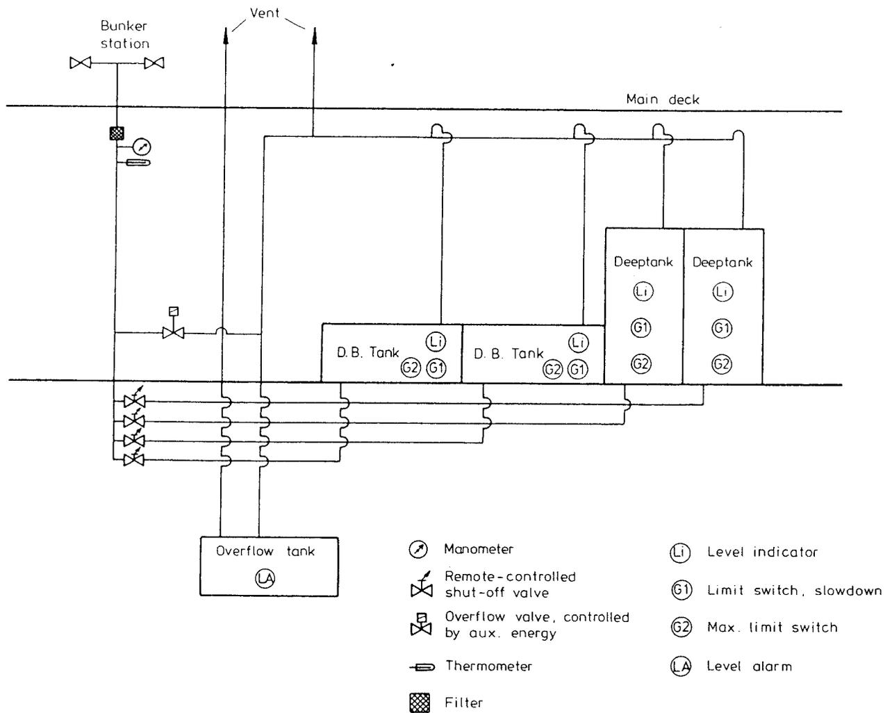
Fig. 3 Fuel Oil Overflow System of Group III
