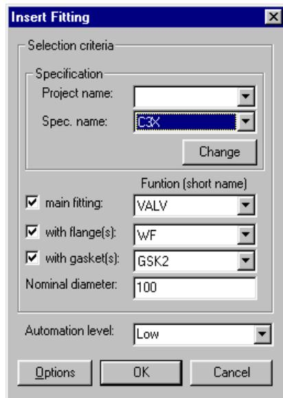
Example of selection criteria for finding fitting component, including flanges and gaskets.
