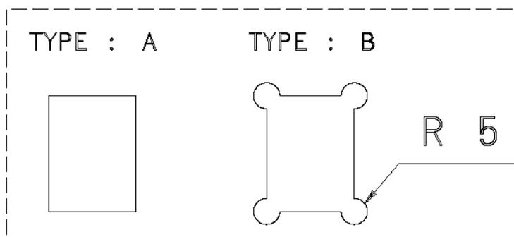
Standard and general holes can be created in all profiles but this automatic function is only valid on L, T, F, I –bar.
