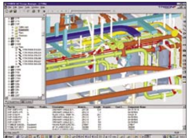
3D view of the Tribon PIM with the parts list window active.
