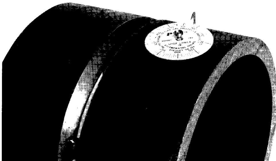
Figure 39—Surface Contact Thermometers
