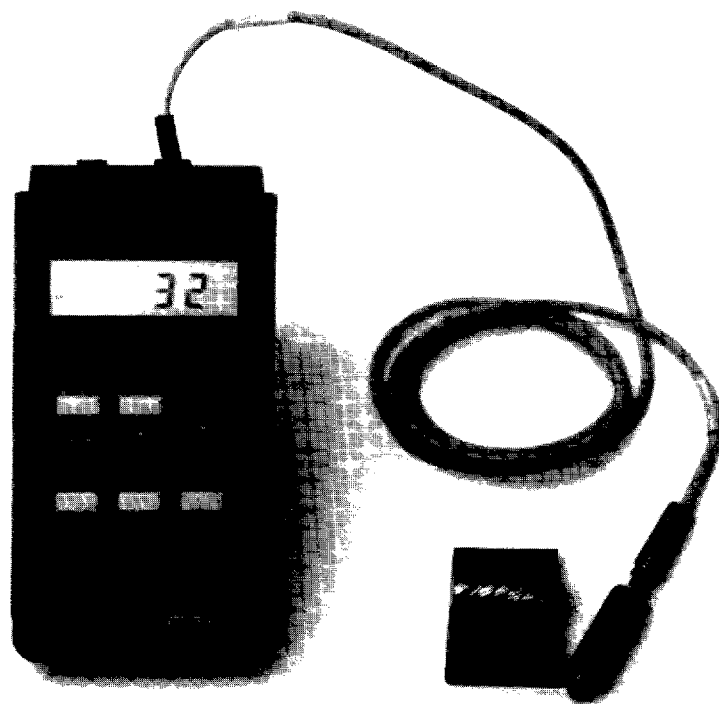
Figure 47—Ferrite Indicator (Ferritescope)
