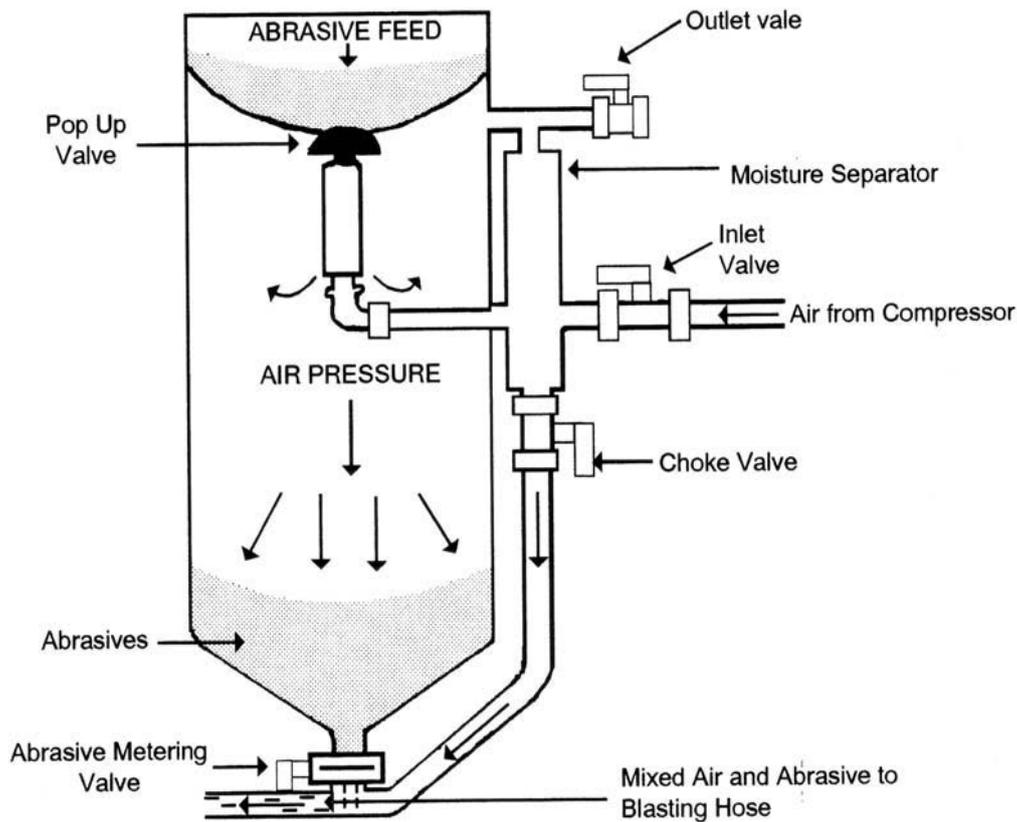
Abrasives are fed into the top of the pot, past the internal pop-up valve, when the machine is depressurized. The abrasives can be stored in a hopper feeding directly into the pot, or they can be emptied into the pot manually by a 'pot man'. When the pop-up valve is closed, compressed air which has been fed through a moisture separator via an inlet valve, pressurizes the section of the machine containing the abrasives.
