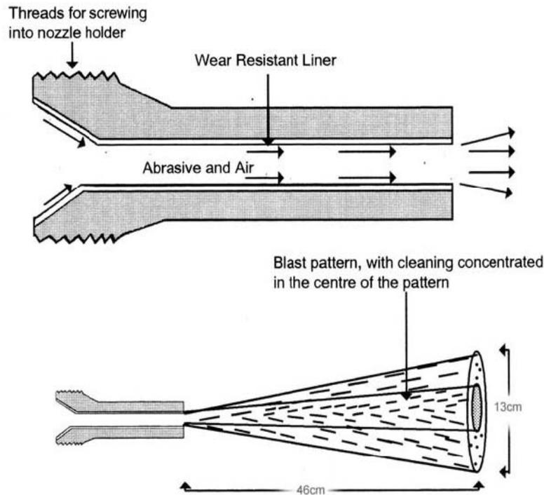
Straight bore nozzles are not widely used now. They have a sharp converging angle into the nozzle orifice, which leads to the straight section of the nozzle. This does **not** flare out towards the outlet end and it gives the abrasive a velocity of about 354 km/h (220 mph) with  $7 \text{ kg/cm}^2$  (100 psi) blast pressure.
