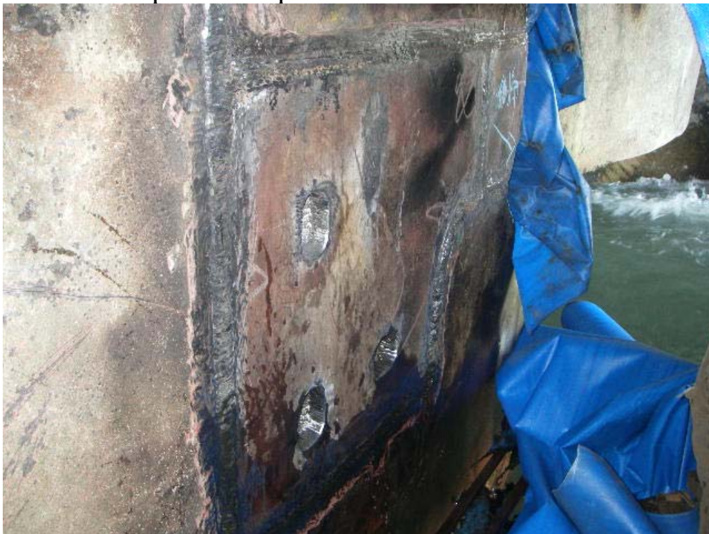
Rudder side plate after plates inserted
