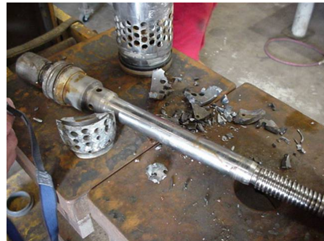
Subsea Production Choke Failure
