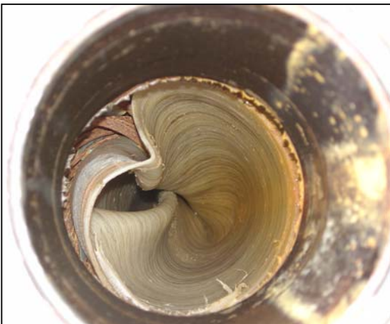
Smooth-Bore Flexible Riser Failure
