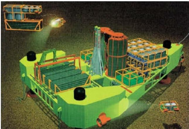
Phase I concept as the diagram shows, was not as radical as expected. The design developed essentially a submerged jack-up rig, that would be controlled and supplied with electrical power from a dedicated surface vessel. Umbilical's would supply necessary compressed air for buoyancy and
