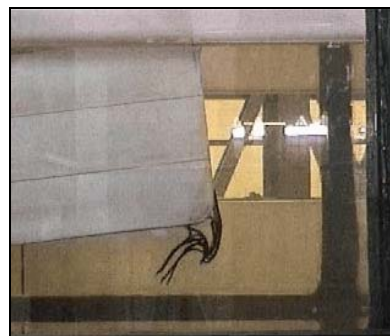
Figure 3 – Visualization of the bilge keel vortex formed by a VLCC mid-ship section box rolling is a decay test; first stages (larger region angles) from Pinheiro [12] and Oliveira [13].
