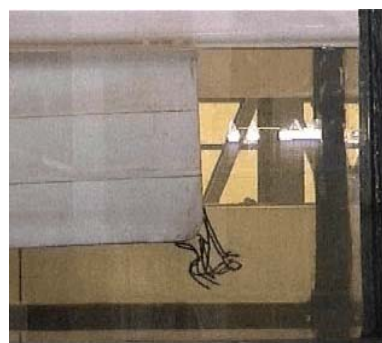
Figure 4 – Visualization of the bilge keel vortex formed by a VLCC mid-ship section box rolling is a decay test; later stages (smaller region angles) from Pinheiro [12] and Oliveira [13]; the vortices form a sidewise 45° street - see Figure 6.
