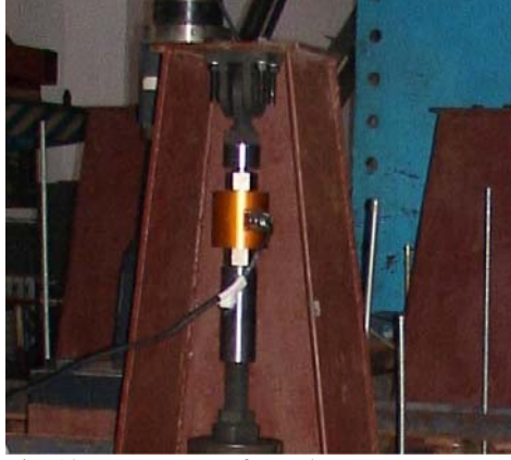
Fig. 10 Force sensor of MR damper
