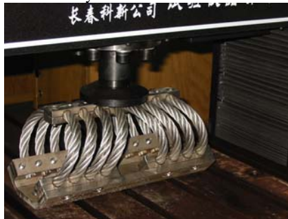
Fig. 6 Steel rope spring in calibrating test
