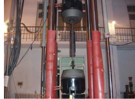
Fig. 4 MR damper in calibrating test
