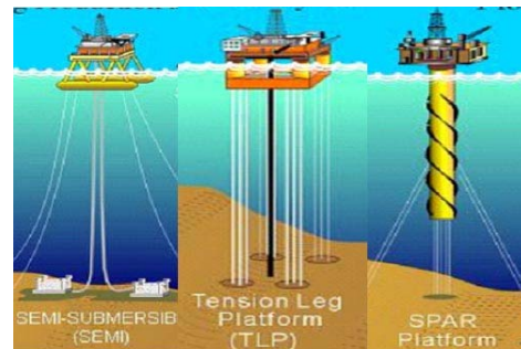
Figure 1: Sketch of SEMI, TLP and Spar
