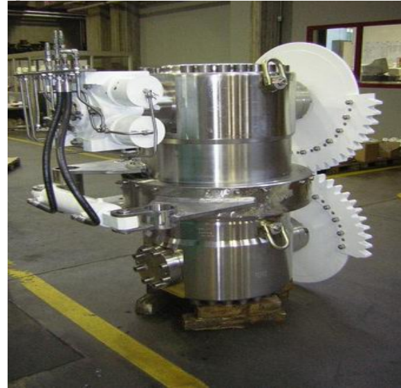
Figure 6: Hydraulically Operated Riser QC/DC Valves
