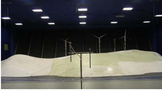
Figure 3: Reproduction of full-scale wind farm in the wind tunnel
