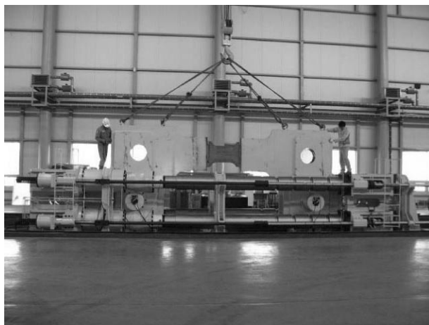
Fig.11 Large tensile test specimen and 3 000 t tensile testing machine
