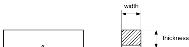
Fig. 4 Charpy V-notch test piece.
