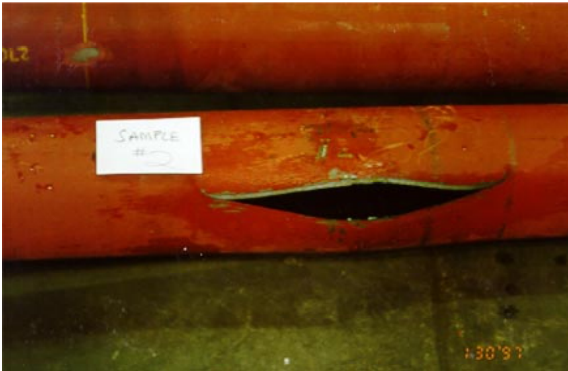
Figure A-1—Ductile Burst Sample
