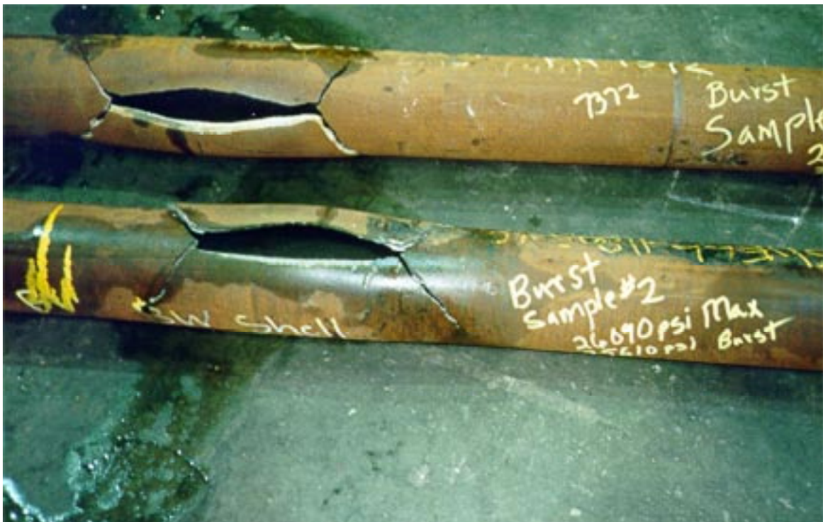
Figure A-2—Brittle Burst Sample
