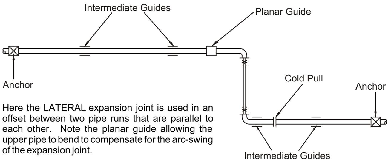
Here the LATERAL expansion joint is used in an offset between two pipe runs that are parallel to each other. Note the planar guide allowing the upper pipe to bend to compensate for the arc-swing of the expansion joint.
