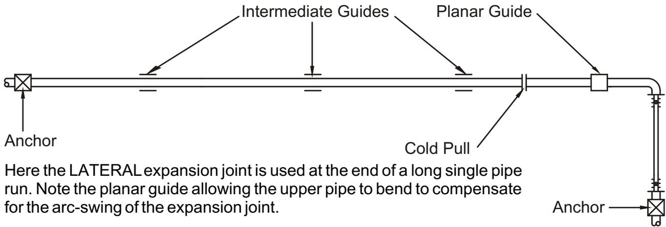
Here the LATERAL expansion joint is used at the end of a long single pipe run. Note the planar guide allowing the upper pipe to bend to compensate for the arc-swing of the expansion joint.
