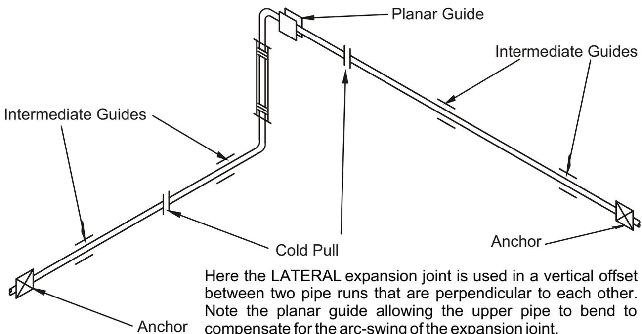
Here the LATERAL expansion joint is used in a vertical offset between two pipe runs that are perpendicular to each other. Note the planar guide allowing the upper pipe to bend to compensate for the arc-swing of the expansion joint.
