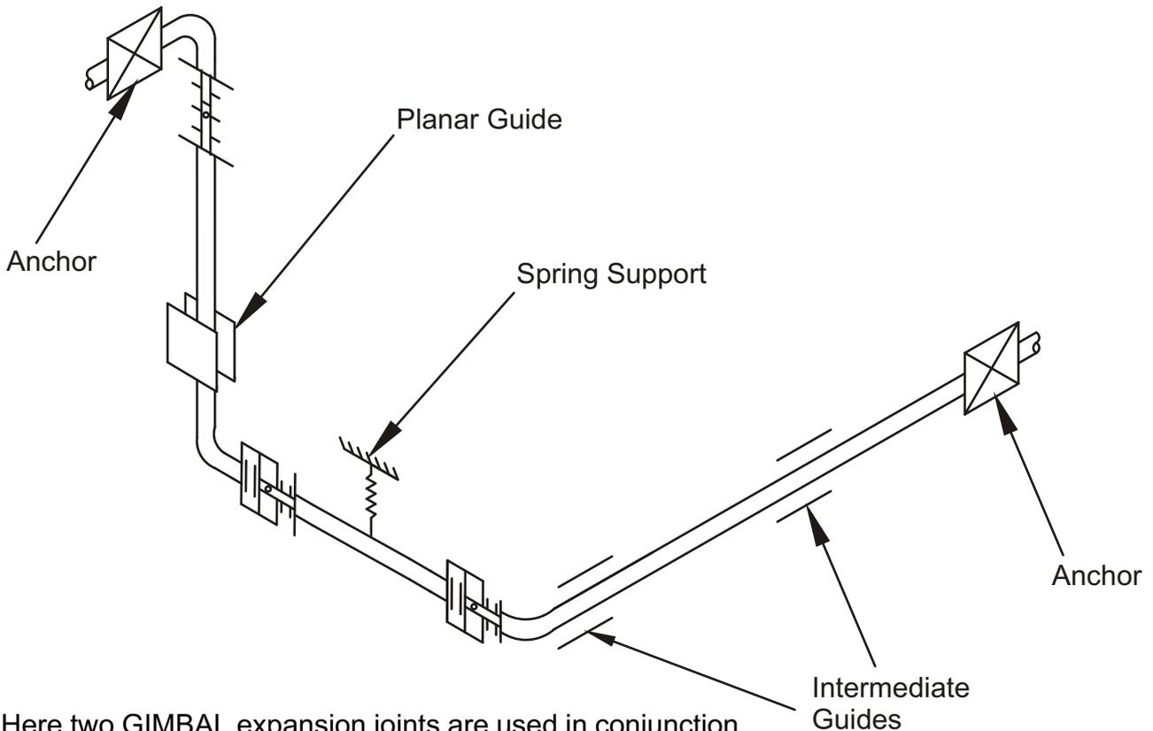
Here two GIMBAL expansion joints are used in conjunction with one HINGED expansion joint to accommodate thermal expansion in a complex multi-directional pipe system.
