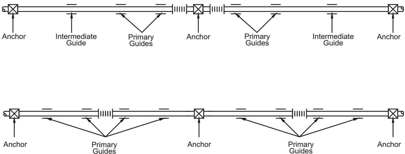
The same comparison with regard to the numbers of guides can be made for the above two diagrams. Also consider in these two cases the ease of access for periodic inspection in the future; i.e. one access point, or two access points.
