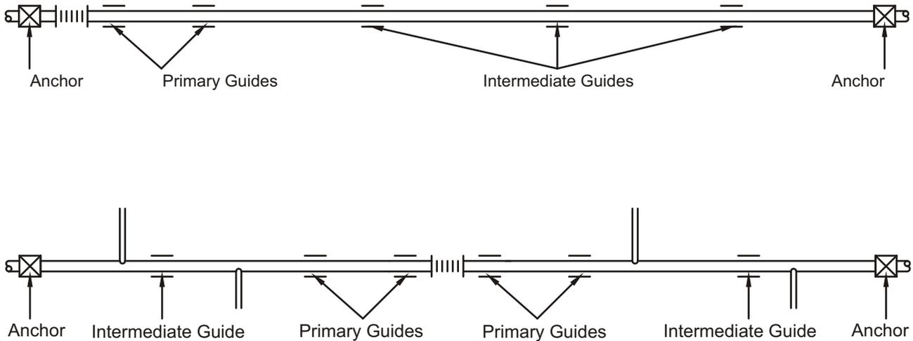
Comparing the two diagrams above, it can be seen that the axial expansion joint may be positioned anywhere in a straight pipe run. However, the number of primary and intermediate guides required varies, so it is important to carefully consider the options available on site.
