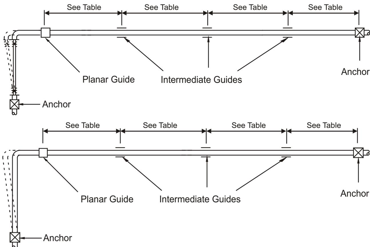
When considering pipe guides for use with restrained expansion joint systems or natural flexing pipe systems, the spacing depends on the pipe nominal size, material, wall thickness and forces acting along the pipe.
