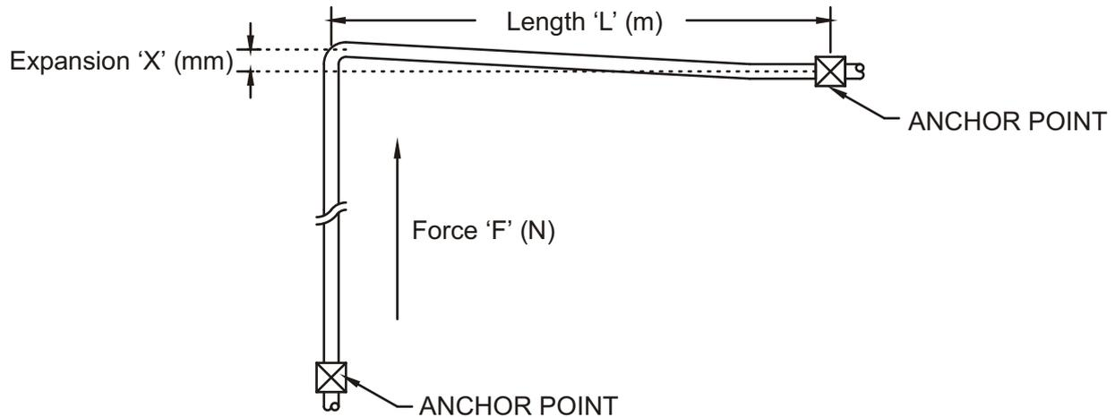
The length of pipe required to bend can be calculated mathematically using the formulae:-
