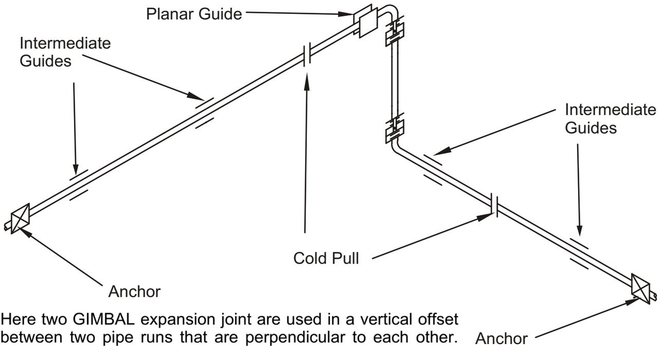
Here two GIMBAL expansion joint are used in a vertical offset between two pipe runs that are perpendicular to each other. Note the planar guide allowing the upper pipe to bend to compensate for the arc-swing of the expansion joint.
