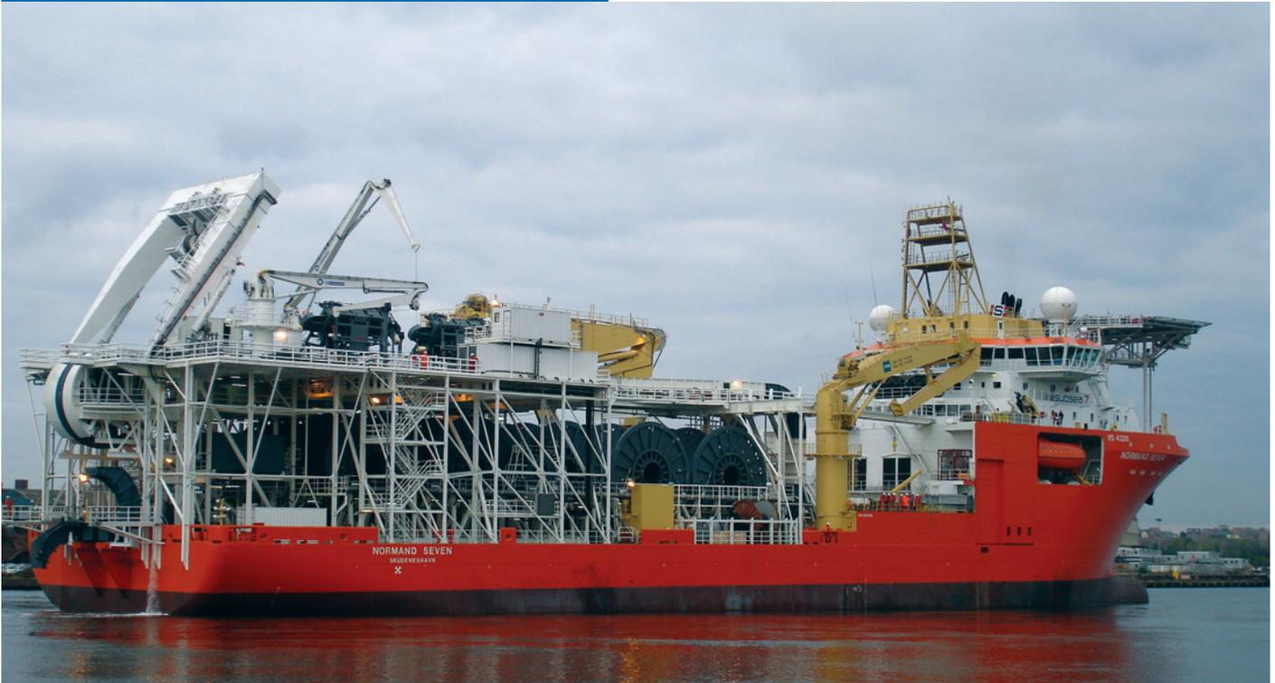
The Normand Seven is a state-of-the-art subsea pipelay vessel fitted with an advanced flexible pipelay system capable of operating in water depths of up to 2,000 m with a top tension capacity of 300 t.
