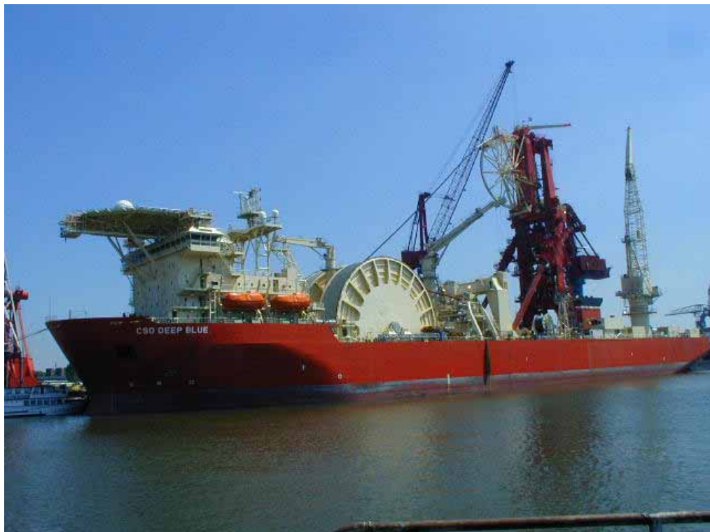
Figure 6-4: Technip Deep Blue Installation Vessel – Reel-Lay and J-Lay
