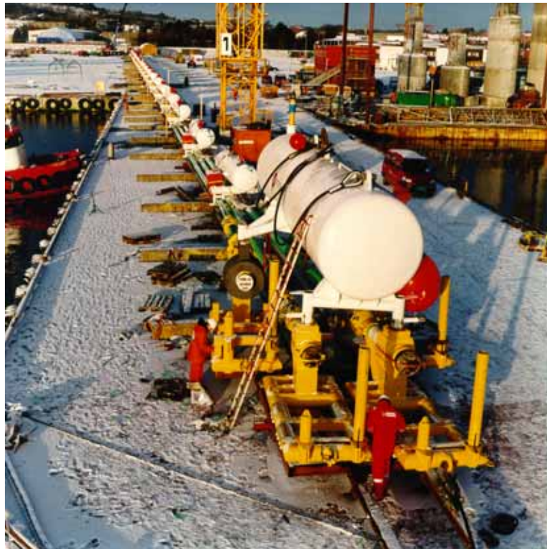
Figure 6-5: Fabricated Riser Bundle System at Yard
