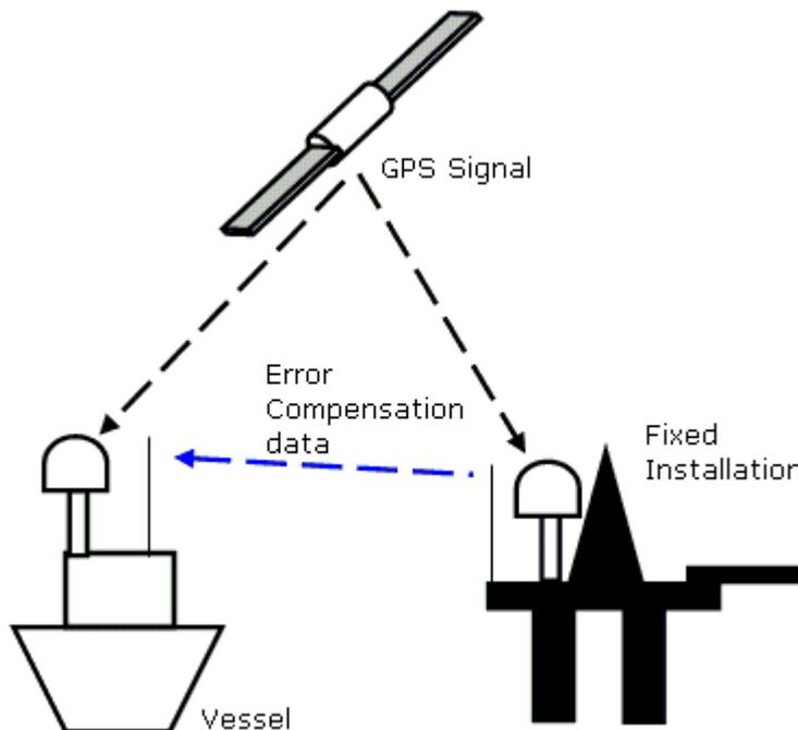
A satellite signal is received by both the vessel and by an installation whose position is precisely known. Any error in the signal from the satellite is converted into an error correction signal which is then broadcast. This signal is received by the vessel, a calculation is made and a more precise position now known.
