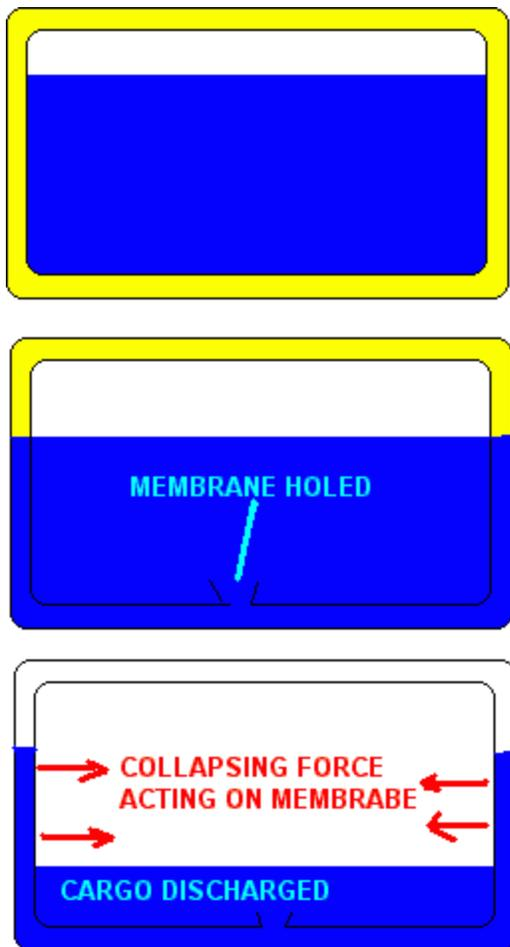
Should a leak be detected from the tank into the interbarrier space by either temperature probes or gas detectors during the loaded voyage the inter barrier space will fill to the level of the liquid in the tank. On discharge it is possible that the level in the tank will fall more rapidly than the liquid can drain from the inter barrier. The primary barrier, which has little mechanical strength will thus collapse.
