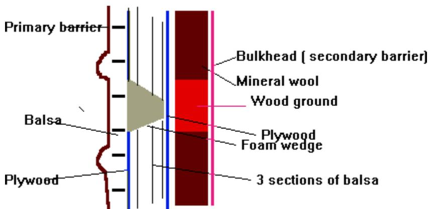
Primary barrier material must have the ability to maintain its integrity at the low temperatures. 36% Nickel steel(invar), stainless steel and aluminium are satisfactory at normal LNG temperatures.
