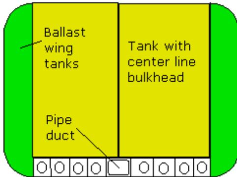
Chemical carriers are basically tanker type structures which are arranged to carry certain types of noxious substances. The structure will generally consist of central cargo tanks with the wing tanks and double bottoms used for dirty ballast. Restrictions will apply if the cargo being carried reacts with water and in these cases void spaces are required. Materials used for construction will depend upon the type of cargo being carried and these are grouped depending upon their properties.
