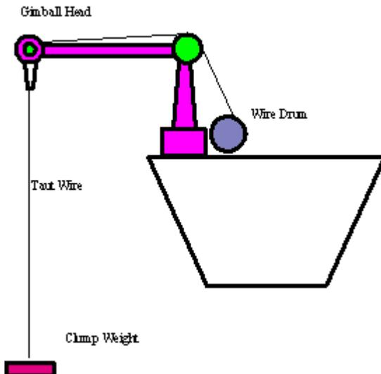
A substantial weight is lowered to the sea bed attached by a high tensile steel wire or minimum diameter ( reduces effect of current).
