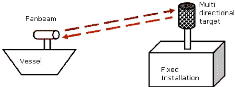
This is an auto tracking system whereby a scanning head fires a laser beam through one lens and receives a reflection of it through a second
