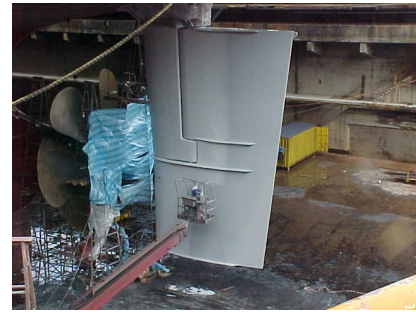
Fig. 11 Scissor Plates on a Semi-Balanced Rudder
