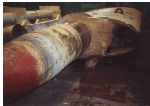
Fig. 6 Profile Thickening in the Pintle Area
