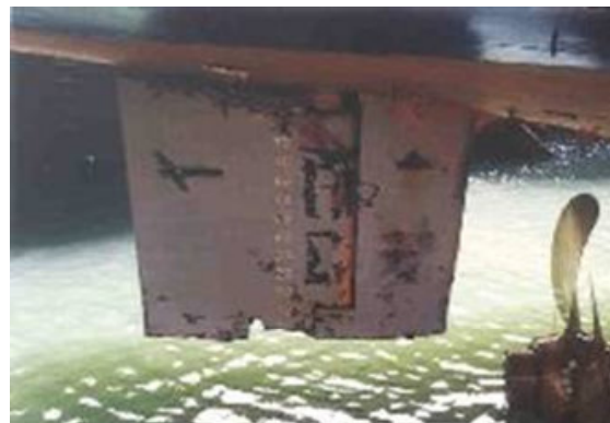
Fig. 1 Damaged Rudder
